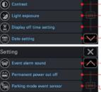
Set up event alarm Set up car battery low power detection Set up impact sensor in parking mode
