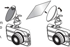
→ Loosen the knob to swivel the device vertically. Locking knob, and confirm that the device is securely locked in place.
