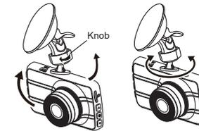
→ Rotating the device to have proper view.
