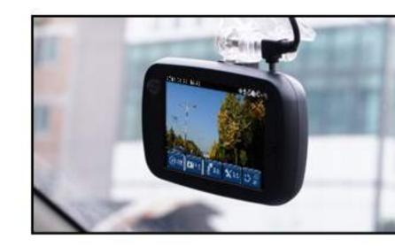
After booting, you can see front and rear view on the LCD screen. Check if it records well and adjust camera angle if necessary.
