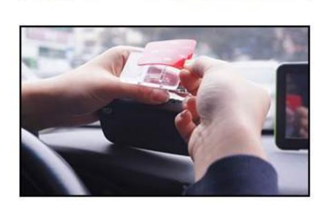
Attach the double sided adhesive tape on the mount holder.
