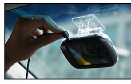
Connect the rear camera into the main camera. Fix the rear camera on the rear window shield, and connect the rear cam cable between rear camera and RCAM port of main camera.
