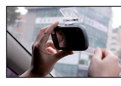
Fix the mount holder onto window screen. In order to avoid affecting driver's sight, it's better to choose a space in the back of room mirror, then adjust camera angle.
