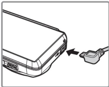
2. Plug the other end of the car adapter to the cigarette lighter socket of your vehicle. Once the vehicle engine is started, the device automatically turns on. Car charger input: DC 12 / 24V.
